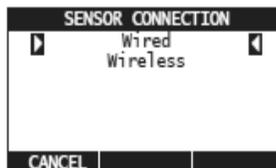
If wired Sensors were programmed via INSIGHT, and wired correctly before Device site installation, the timer does not apply. Select Wired, ← . Next select the output
