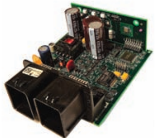
Winland produces this circuit board assembly, part of a sensor system that detects rollover risk in emergency response vehicles and activates seatbelts and airbags. The manufacturer came to Winland a year ago looking for improvements to its existing design.
